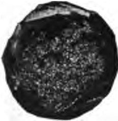
FIG. 24.—Crystalline Fracture of Wrought Iron when broken suddenly.
